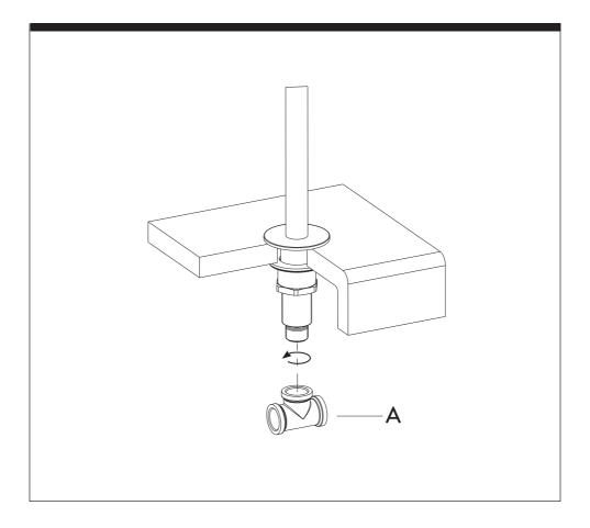
Fit the T connection (A) by screwing it to the lower side of the spout. We suggest to adjust it in the right position to fit then the two taps at its sides.
