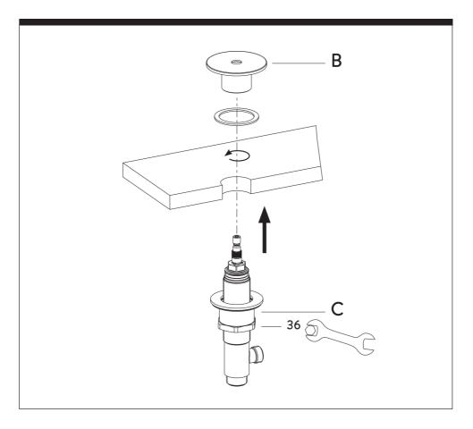
Fit the two standings, fitting it from below and screwing the chrome ring (B) with its gasket, and fix the set with the fixing nut (C).
