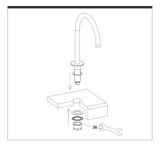
Fit the spout fixing the set with the lower fixing nut and gaskets.
