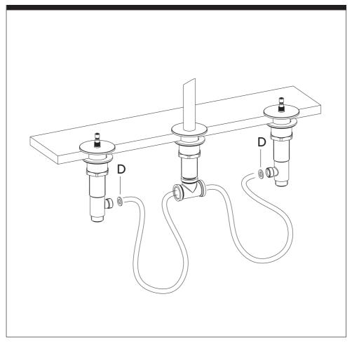
Join the two standings to the "T" connection by mean of the flexible hose supplied and be careful to fit the gaskets (D).
