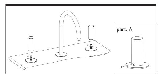
Finally fit the two handles and fix them with their grub screws (see part. A).
